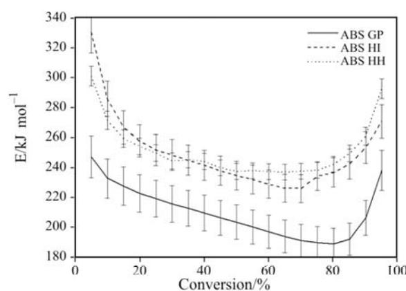
Fig. 7 Activation energy ( $E$ ) of ABS using the model-free kinetics
