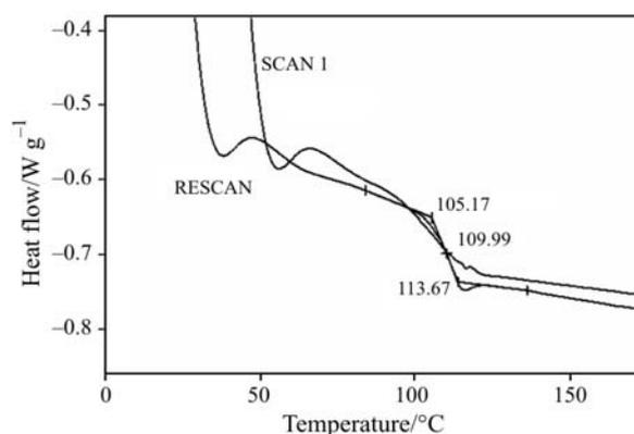
Fig. 2 DSC curve of ABS HI (onset  $T_g$ =105.2°C)
