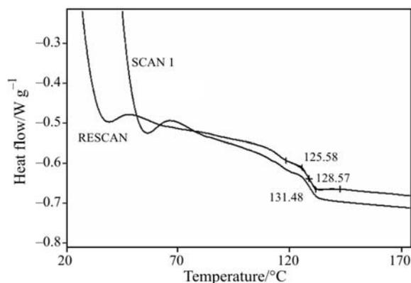
Fig. 3 DSC curve of ABS HH (onset  $T_g=125.6^\circ\text{C}$ )
